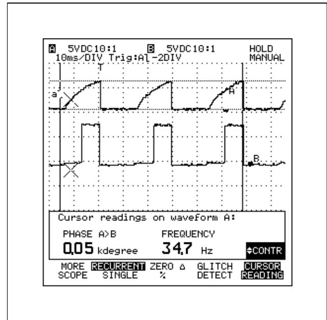
Figure 8-20 Phase Measurement
