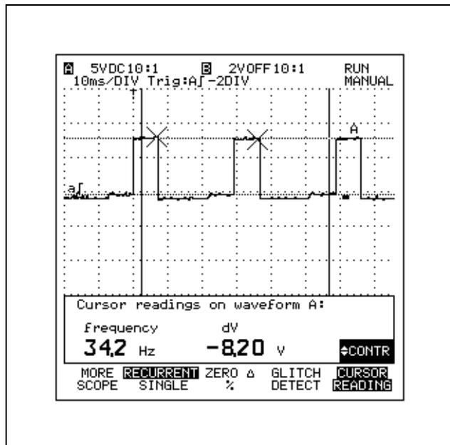
In this example, the markers are defining sample points for measuring frequency.
