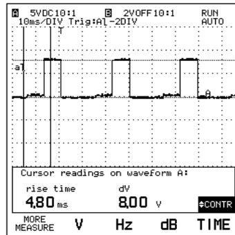
10.   The left and right cursors move across the display. The intersection of waveform and cursor mark the level for the two horizontal cursors.
