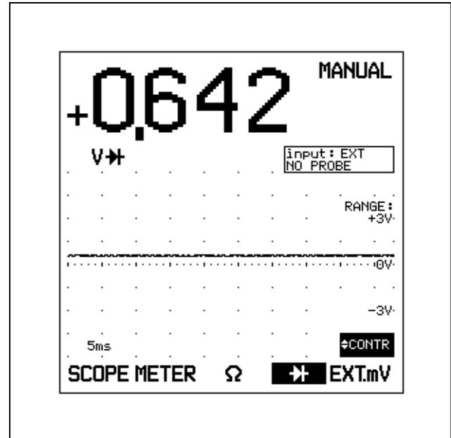
**F5** **EXT.mV** EXTernal milliVolt function. Signals supplied to the red and black 4-mm banana jack inputs are measured. The red banana jack is the high input, and the black banana jack (COM) is the low. The ranges are 300 mV, and 3V. Time base ranges are from 1  $\mu$ s to 100 ms/div.
