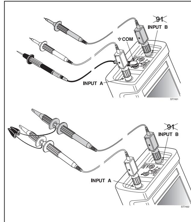
Figure 5-1 Scope Connections
