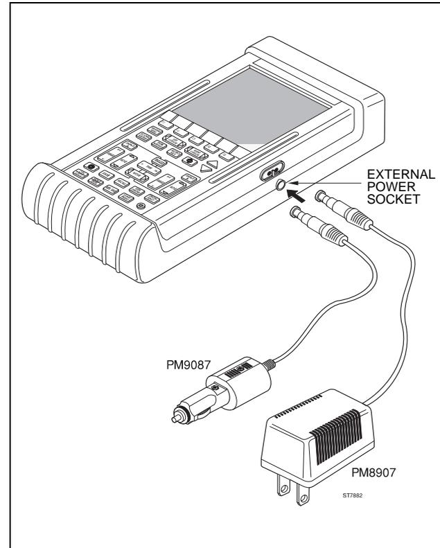
Figure 1-2 Power Connections
