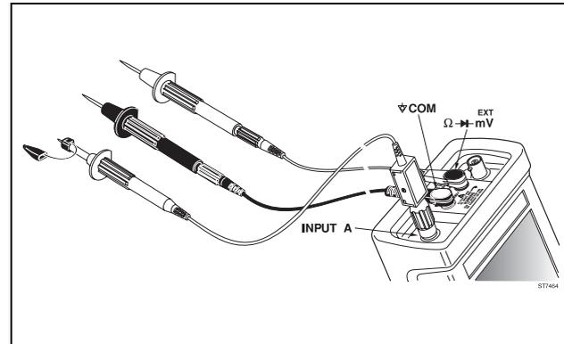
Figure 3-1 Measurement Connections
