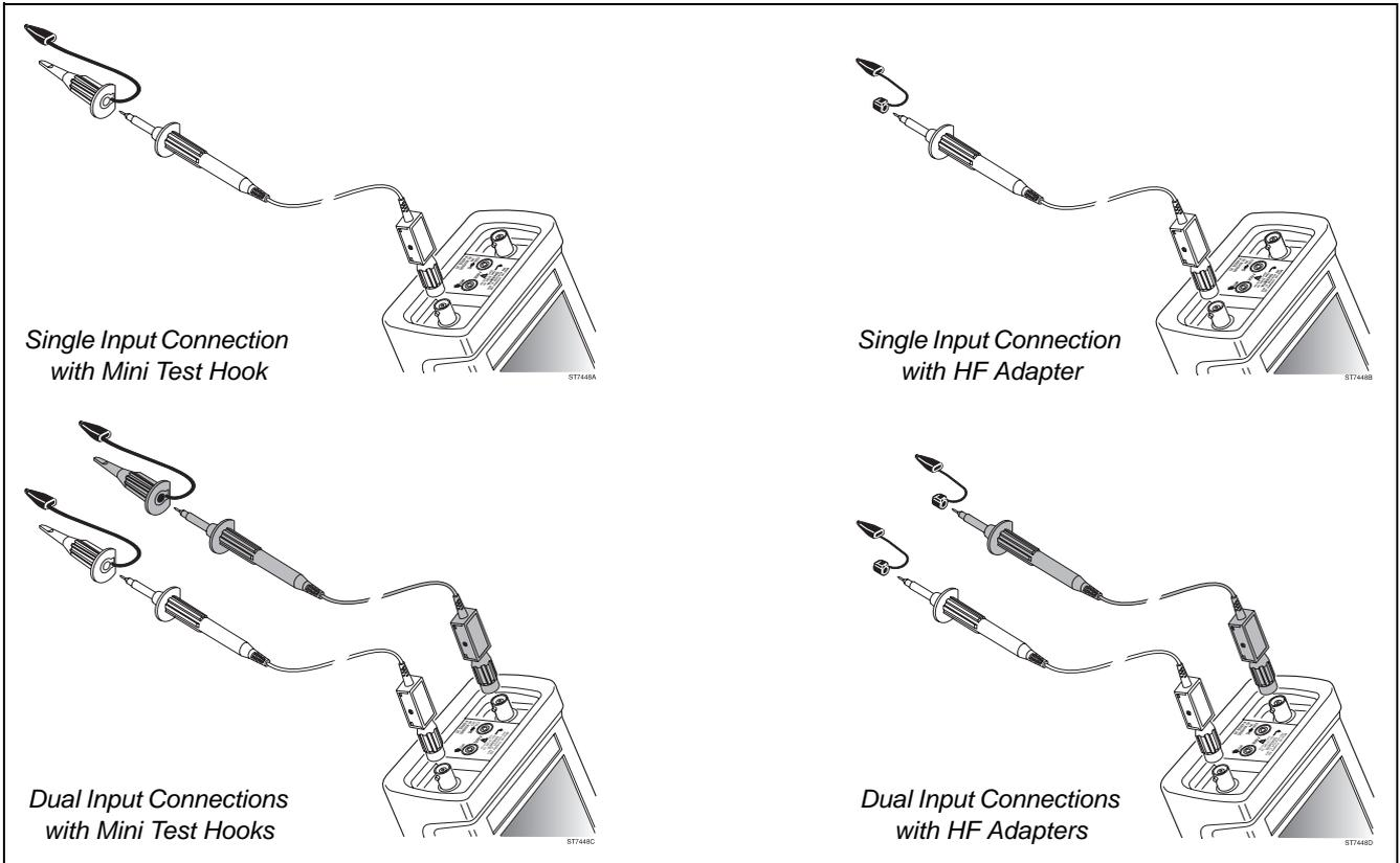
Figure 3 Input Connections for High Frequency Electronic Measurement
