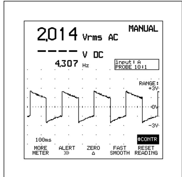
Figure 8-6 Vrms AC Display in Meter Mode
