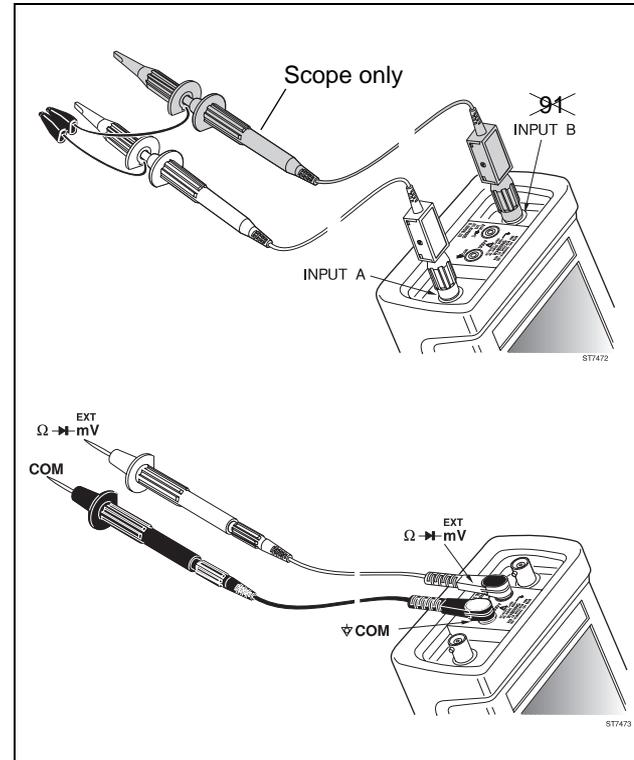
Figure 4-1 Measurement Connections
