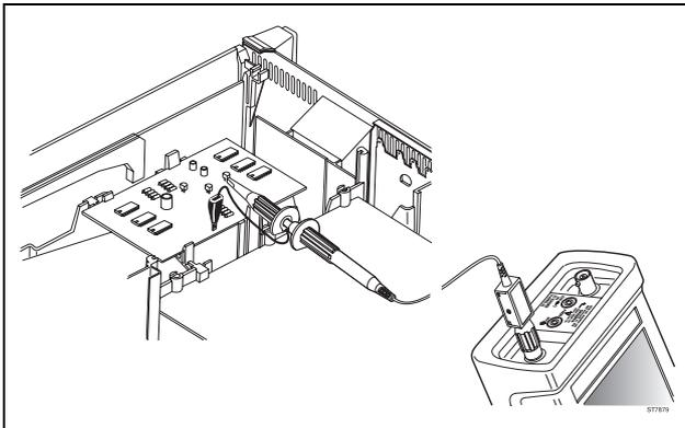
Figure 7-13 Measuring the rise time of a pulse.
