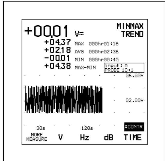
Figure 8-4 MIN MAX Recording with Trend Plot Function
