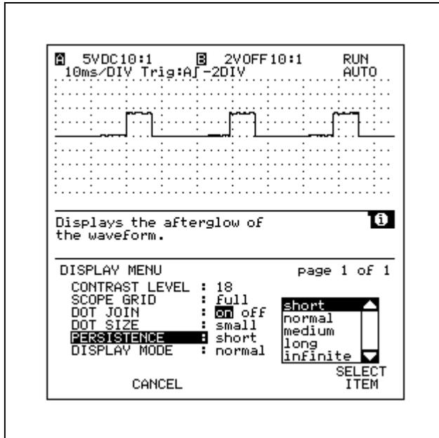
In the DISPLAY window you can also choose the DOT JOIN function, which either shows the individual measurement samples or joins them together to give a continuous trace.
