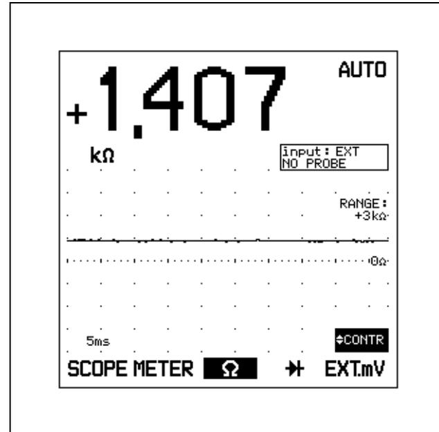
The measurement result is displayed as a 3 2/3-digit display. The ranges are 30 $\Omega$  (manual only), 300 $\Omega$ , 3 k $\Omega$ , 30 k $\Omega$ , 300 k $\Omega$ , 3 M $\Omega$ , and 30 M $\Omega$ . A beeper alert is generated at <5% of a selected range in Manual Range mode. The beeper alert is turned on with ALERT))).
