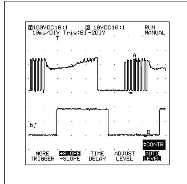
Figure 8-11 PWM Motor Drive Signals
