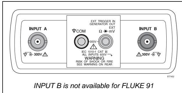
Figure 1-3 Measurement Connections
